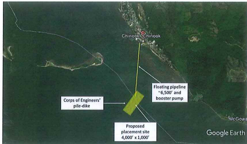
Figure 11. Port of Chinook Disposal Alternative 2 schematic
