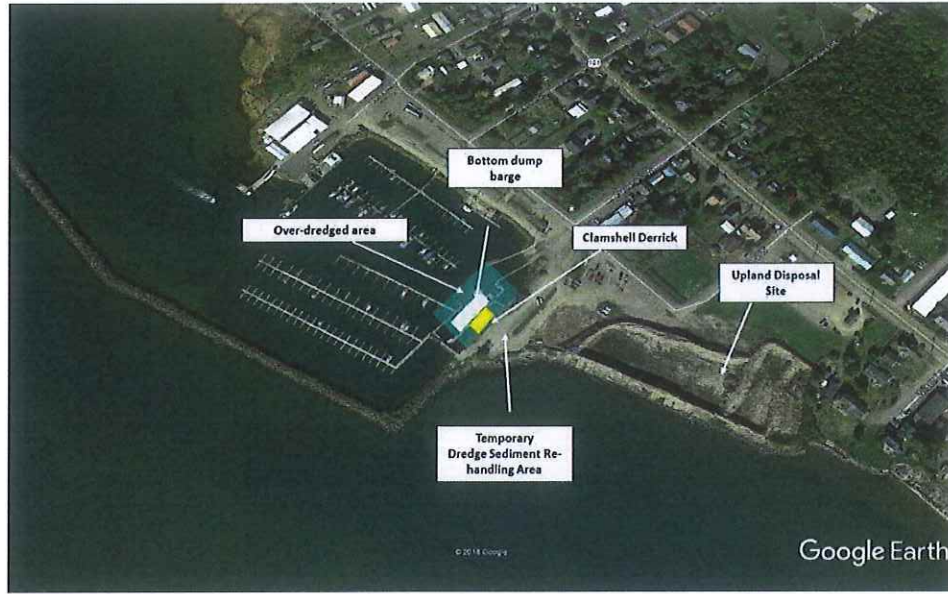
Figure 10. Port of Chinook Disposal Alternative 1 schematic
